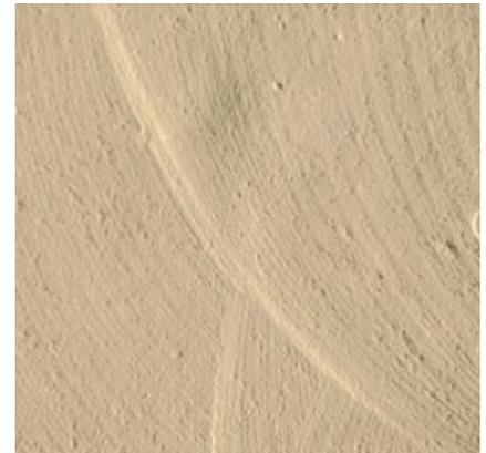
**ICRI's CSP-2 (left) and CSP-3 (right) profiles shown are the most commonly specified surfaces for surface membrane systems.** PHOTO: JOE NASVIK
