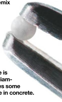
polymer beads have negligible water absorption and concrete made with them can be easily pumped at water-cement ratios of 0.40. Drying rates for concrete made with Elemix closely match rates of normal weight concrete, though quicker drying can be achieved.
