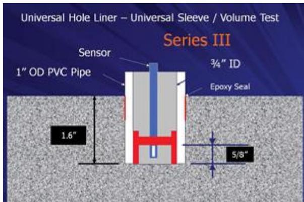
Based on the results of this study, the ASTM F 2170 test method was rewritten in 2011 with a stronger emphasis on the hole liner totally isolating the measurement to the bottom of the drilled hole. Also, moisture from the target depth would not be allowed to migrate outside of the hole liner or to a height greater than 5/8 inches inside of the liner.
