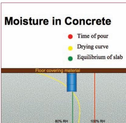
Once a floor covering is installed, the relative humidity equilibrates throughout the slab (green line). Taking readings at 40% depth (slab on grade) prior to installation of a floor covering tells us what the slab will eventually equilibrate to after the floor covering has been placed (intersection of yellow and green line).
