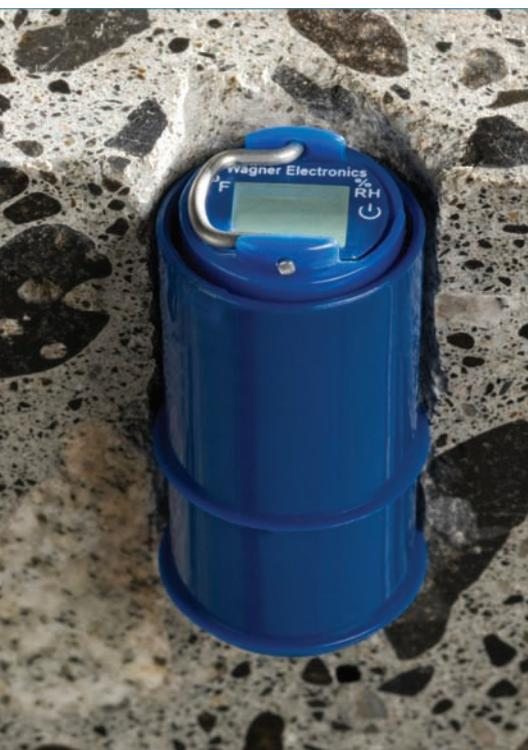
The Wagner Electronics Rapid RH™ Smart Sensor is 3/4" in diameter, and measures both temperature and relative humidity within the slab.
